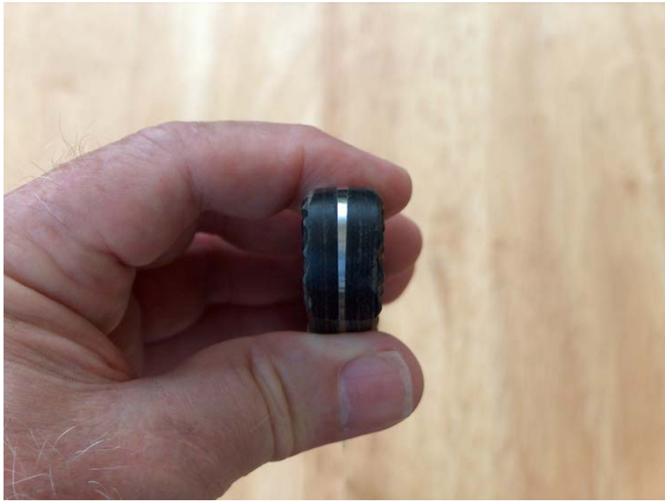
Butt end of handle showing tapered stock that comes already thicker at the spine and thinner for the edge for stock removal makers
