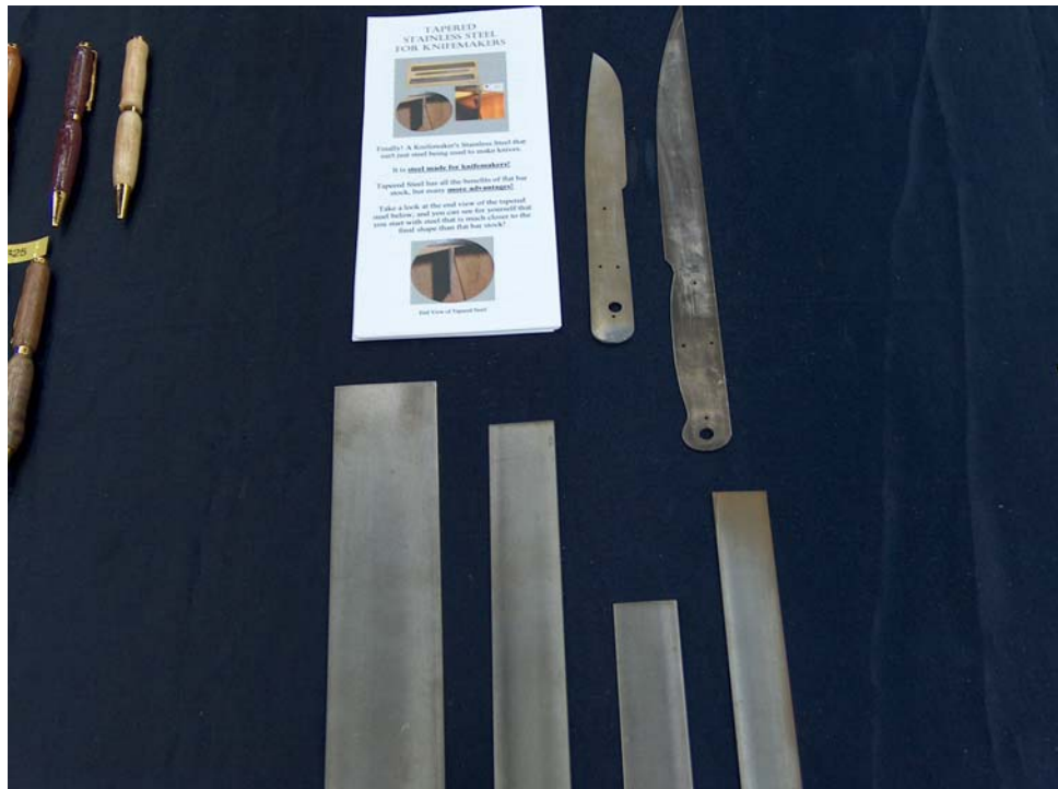
Display of tapered stock 420 modified steel distributed by Robert Fisher at the 2007 Blade Show
