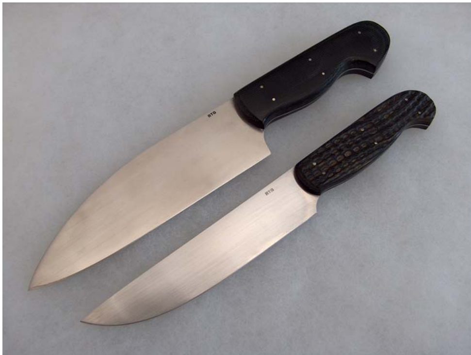
Test knife number 1 (top) made 850 slices of rope. Subsequent knife (bottom) made 100 slices of rope. The steel and edge geometry were the same. What caused the cutting performance difference? See text.
